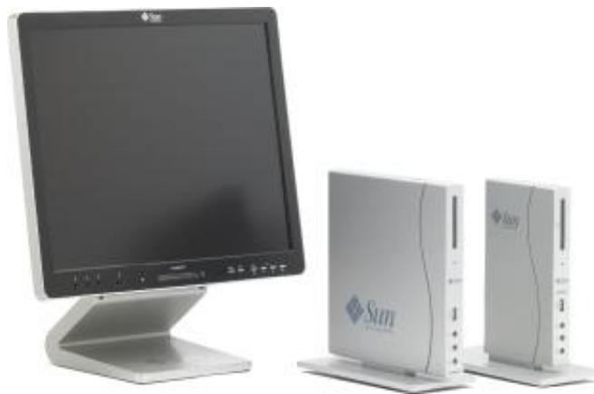
Figure 7 The Sun Ray 270, 2FS, and 2 thin clients (from left to right)
